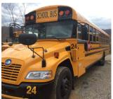
ginia requires three warnings for low air brake pressure, including the highly visible wig-wag device, which had not been seen on state school buses since the late-1970's.
